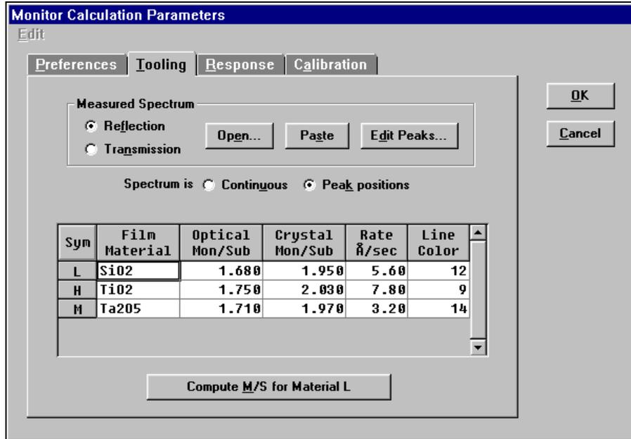
Materials listed in the **Film Material** column can be printed in the coating run-sheet. The **Rate** column helps MONITOR provide a more realistic strip-chart simulation graph. This grid also includes a **Line Color** column for assigning colors for the strip-chart simulation.
