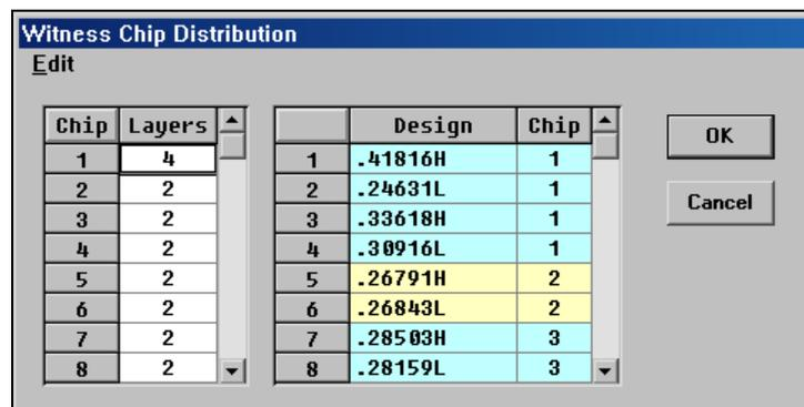
Click **Setup...Chip Distribution <Ctrl+H>** to specify or change the number of layers on each chip. (The dialog box is automatically activated after loading or
