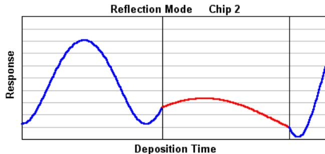
A far more dramatic change occurs in chip 2. The cutoff for layer 2 now utilizes its own maximum as well as the previous minimum from layer 1. The cutoff for layer 3 uses its minimum as well as the previous maximum from layer 2.
