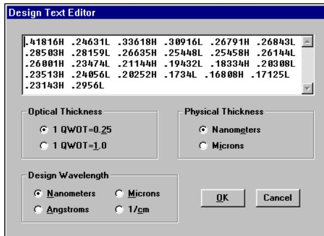
A design containing parentheses, *i.e.* (.125H .25L .125H)10, is 'exploded' into individual layers upon returning to the Layers Editor. Adjacent layers of the same type are combined when there are parentheses. That is .125H .125H becomes .25H. (Adjacent layers are NOT combined in the Layers Editor. This makes it possible to break up thick layers into thinner layers of the same type.)
