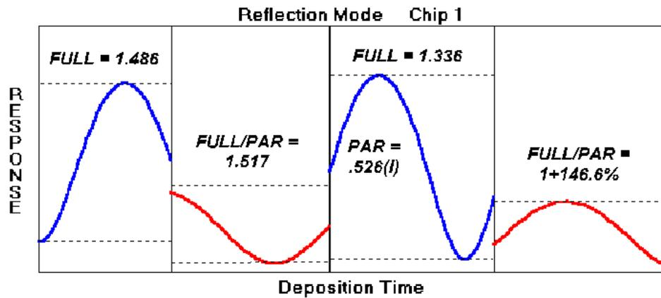
**FULL Swing**...An integral full swing encompasses the complete maximum to minimum excursion. Referring to the diagram, layer 1 response starts at the minimum value, rises to its maximum and finishes at some intermediate final value. In practice, the coating technician counts the number of chart divisions corresponding to the integral part of the swing. That number is multiplied by 48.6% and subtracted from the value at the maximum. That is
