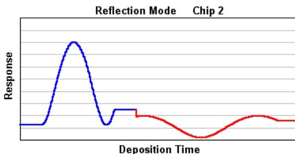
While design layer 4 (C2/L2) has good selectivity, a higher gain setting will be beneficial. Click **Edit...Options** <Ctrl+O> to bring up Worksheet Calculation Options (no need to leave the strip-chart dialog!) and uncheck **Same gain/offset for all layers on chip** to enable variable gain settings (different values for different layers on a chip) and note that **Use current worksheet values** option is now enabled. Finally, change **Auto Level Type** to Initial.
